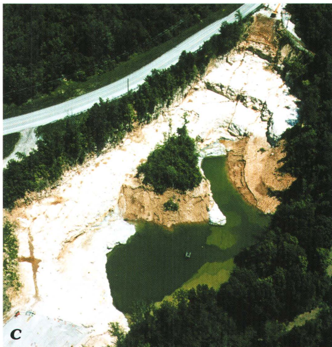
Figure 13. Quarry at Weldon Spring, Mo. Photographs courtesy of Morrison Knudsen Corporation, St. Charles, Mo. A, B , The visual effect of dumping operations from 1940's to 1960's. Waste types included TNT/DNT, thorium, radium, and uranium. C , Excavated quarry basin.
